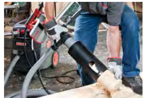
DRILLING IN WOOD with dust extraction – hand-held
