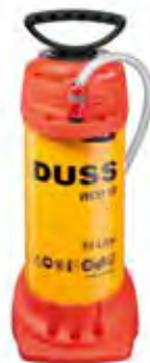
WATER SUPPLY UNIT for use where no water supply is available, steel tank, capacity 10 l, reinforced hose 2.5 m and 1/2" coupling with water stop ORDER-NO. WDB 10
