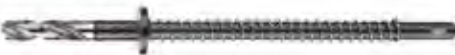
PILOT DRILL BIT WITH EJECTOR drilling dia. 14 mm, overall length 300 mm, the drill core is automatically ejected from the LS core cutter and captured on the tip of the pilot drill bit ORDER-NO. LSZ 1
