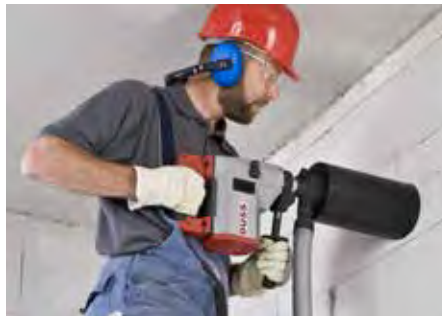
DRILLING IN MASONRY with dust extraction – dry, hand-held
