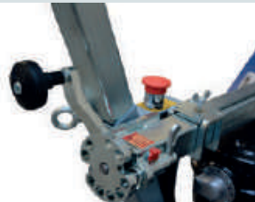
Depth gauge with interlock
