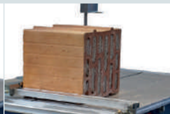
Mineral rock wool filled porous brick
