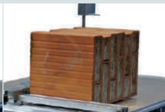
Perlite filled porous brick
