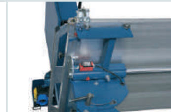
Automatic saw shut-off
